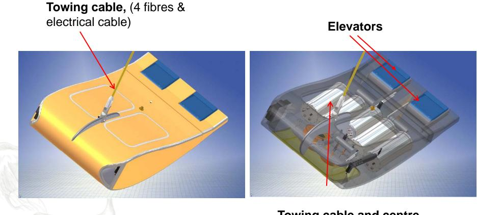
Towing cable and centre plate with fastening holes
