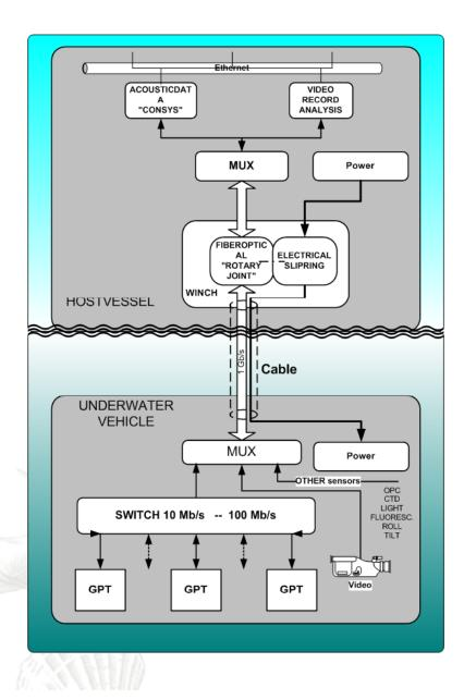
System diagram as blocks and data flow
